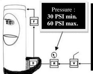
3. Install the bottleless components in the order of the diagram above (V=shutoff valve, R=regulator, D=leak detector, F=filter). Check each component to make sure it is operating properly including putting the water line under pressure to check for possible leaks at each connection point.
