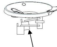
• Before putting the float assembly on the reservoir, make sure that the tube in the center of the cooler reservoir isn't blocking or impeding the mechanism and operation of the float arms. Make sure the water level in the reservoir is low enough not to engage the upper float (safety float).
