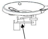
• Release the lower arm, then raise the upper arm (safety float). Make sure that the flow stops completely. Lower the upper arm to its original position.
